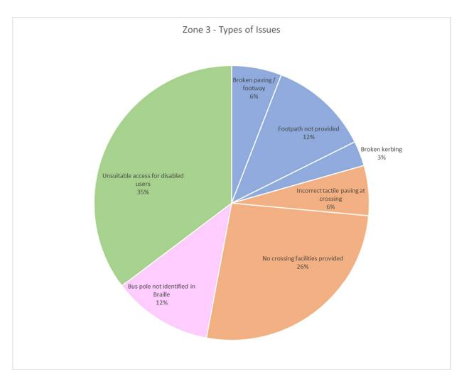
Figure 4.3: Zone 3 – breakdown of types of issues identified
