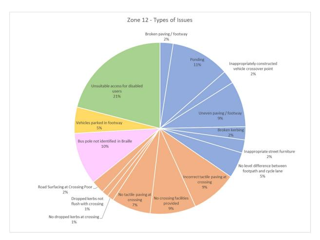
Figure 13.3: Zone 12 - breakdown of types of issues identified
