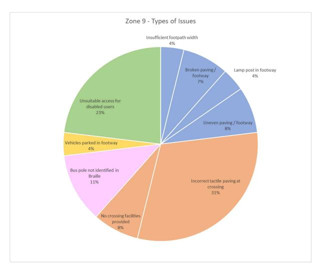
Figure 10.3: Zone 9 - breakdown of types of issues identified
