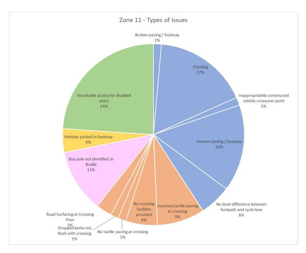
Figure 12.3: Zone 11 - breakdown of types of issues identified
