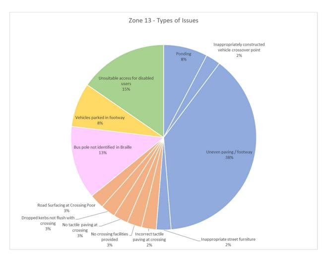
Figure 14.3: Zone 13 – breakdown of types of issues identified
