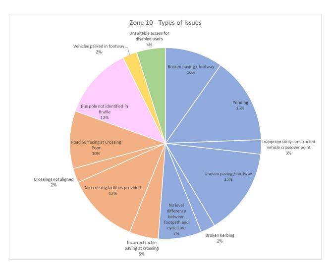
Figure 11.3: Zone 10 – breakdown of types of issues identified
