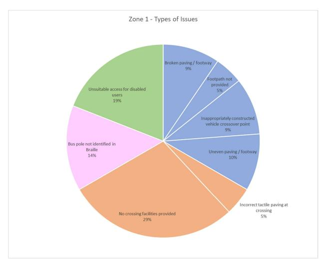
Figure 2.3: Zone 1 - breakdown of types of issues identified
