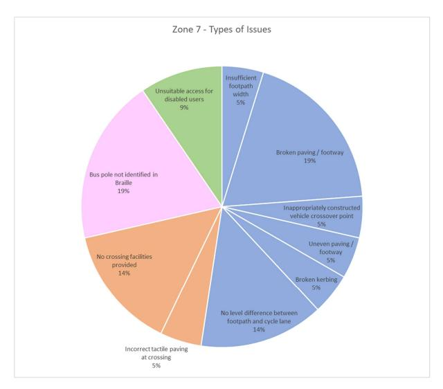
Figure 8.3: Zone 7 - breakdown of types of issues identified
