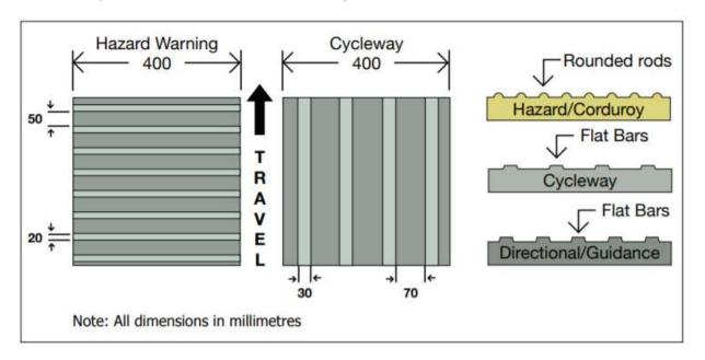
Figure 16.2: Examples of Hazard Warning and Cycleway Paving (Note: Extracted from NDA Building for Everyone: A Universal Design Approach)
